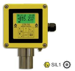
**Gas transmitter GTR 210 MED** is used for the detection of flammable, toxic gases and oxygen in ATEX zone 1.
